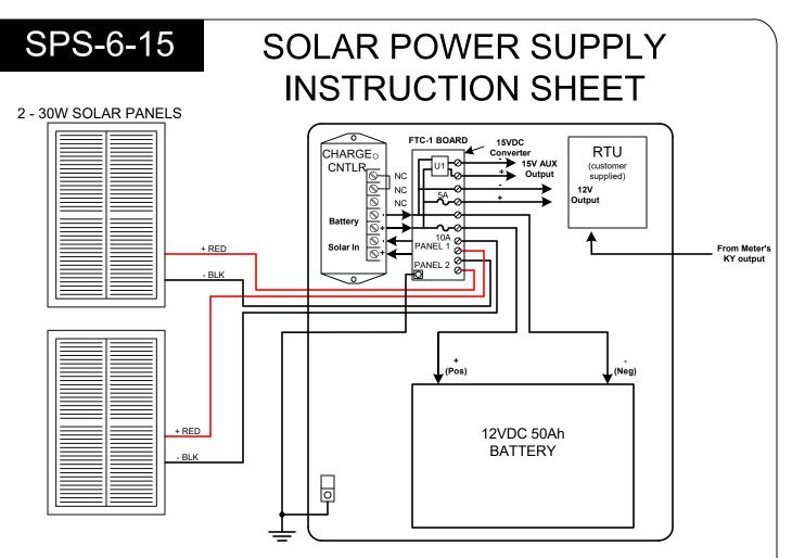
**MOUNTING POSITION** - The SPS-6-15 Enclosure must be mounted in an upright position so that the battery is placed on the <u>bottom</u> of the enclosure. Mount the solar panels using the metal mounting systems provided to get the correct mounting angle pursuant to the instructions included in the mounting bracket kits. The solar panel mounting bracket is designed to attach to a pole or building. Solar Panels may not be shaded by trees or a building at any time.
